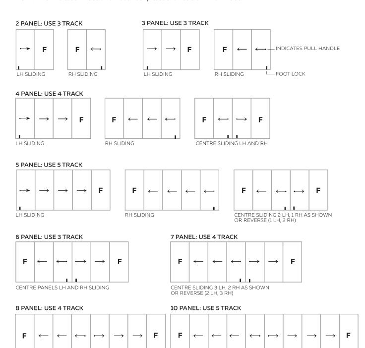
TYPICAL STANDARD CONFIGURATIONS ARE SHOWN. CONTACT LOUVRETEC FOR CUSTOM VARIATIONS
