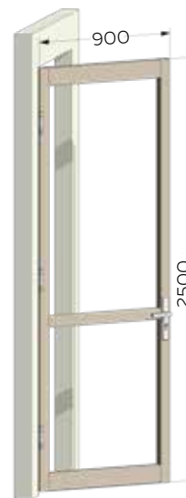
HEAVY DUTY HINGED DOOR RECOMMENDED MAXIMUM SIZE
