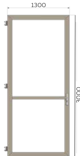
ULTRA WELDED HINGED DOOR – RECOMMENDED MAXIMUM SIZE
