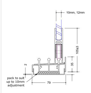
3 PANEL STANDARD TRACK & BASE WITH THREE TRACK ADAPTER CHANNEL
