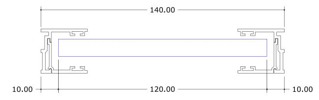
CROSS SECTION WIDTH - GLASS WIDTH = OVERALL WIDTH -20MM
